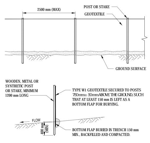
IN UNGRUBBED AREAS WHERE A TRENCH IS IMPRACTICAL, FLATTEN BOTTOM FLAP ON THE GROUND, BACKFILL AND COMPACT WITH SOIL. FLOW  $\sum$ MIN. 150 mm BOTTOM FLAP
