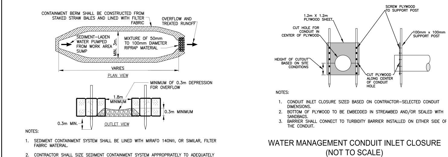
3. CONTRACTOR SHALL INSPECT SEDIMENT CONTAINMENT SYSTEM DAILY AND REPAIR AS NECESSARY TO MAINTAIN SYSTEM PERFORMANCE. ACCUMULATED SEDIMENT SHALL BE REMOVED WHEN STORAGE HEIGHT HAS BEEN REDUCED TO 9 INCHES. REMOVED SEDIMENT SHALL BE DEPOSITED IN AN AREA THAT WILL NOT CONTRIBUTE SEDIMENT TO JURISDICTION AREAS AND CAN BE PERMANENTLY STABILIZED.
