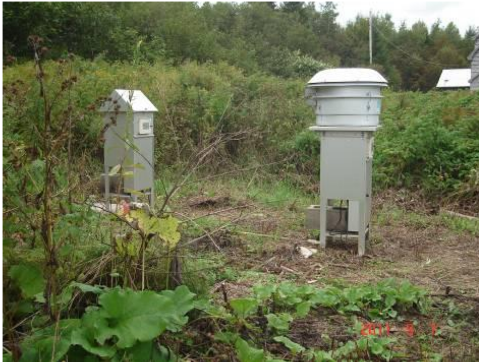
Figure 3.2 Hi-Vol Samplers Monitoring Location – 29 Second Street, Napadogan, NB
