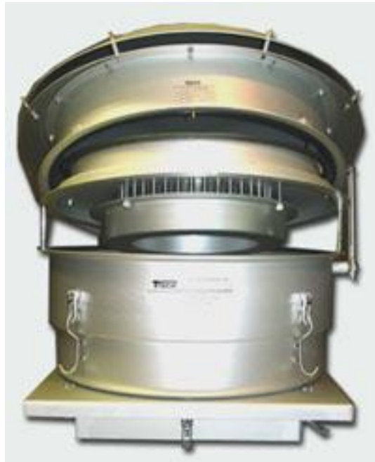
Figure 3.5 PM 2.5 Hi-Vol Selective Size Inlet Sampling Head
