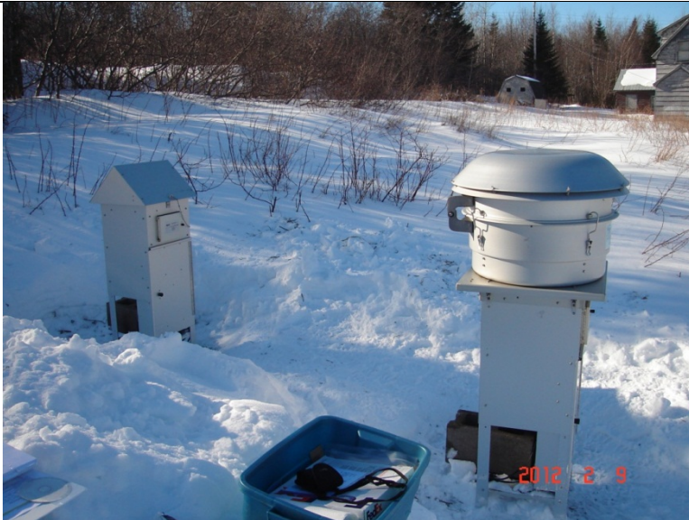
Photo 9 Ambient Air Quality Monitoring Site – Hi-Vols – Winter
