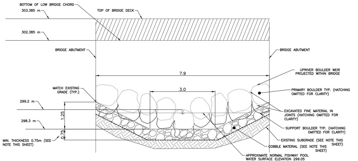
**SECTION VIEW (WATER CONTROL STRUCTURE SECTION)**
