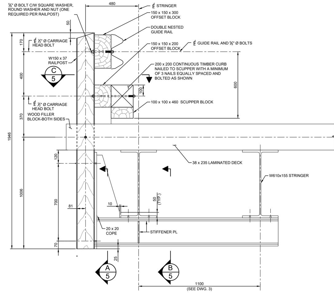
**RAILPOST CONNECTION DETAIL FOR TNL DECK**
