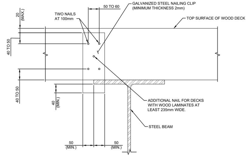
CONNECTION OF NAIL - LAMINATED DECK TO STEEL BEAM
